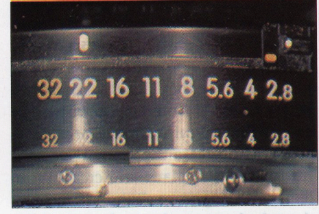
Figure 10. Aperture adjustment setting on the barrel of the lens. Changing the setting (f-stop) opens and closes the internal diaphragm of the lens, allowing in more or less light.
