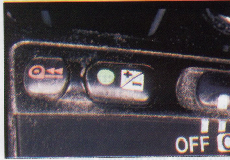
Figures 8a, b, and c. Exposure compensation (EV) controls on a camera are generally labeled “+/-,” either on a simple dial (a) or on a button (b). The dial is adjusted to + or - values to bracket the exposure. Cameras with LCD screens will display the numerical value of the desired exposure compensation in + or - values (c).
